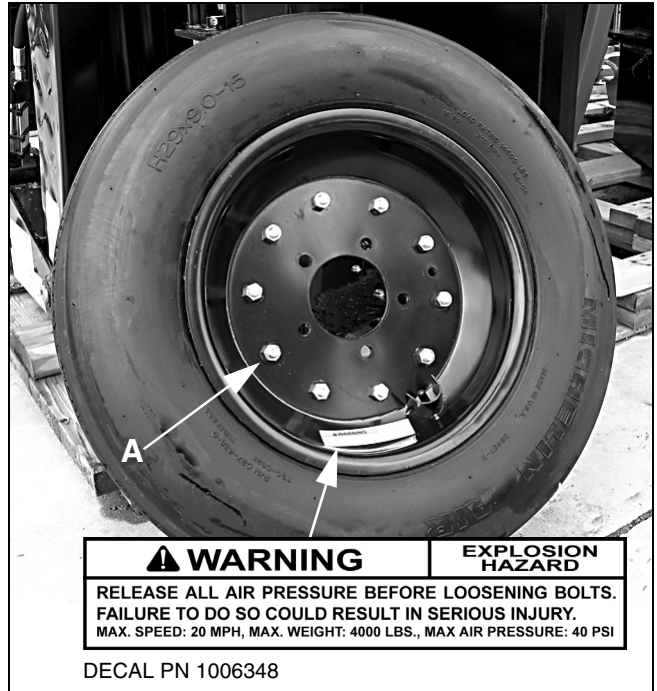
Figure 19. Split Rim Tire Servicing
